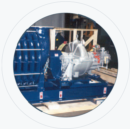
Spencer Power Mizer blowers for installation at an Indonesian plant feature two special drive configurations: one has a steam turbine power source; the other has a motor and gear increaser for use with 50 Hz electricity.
