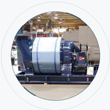
Massive Spencer Power Mizer Series 7000 blower with Acoustical Belly Wrap™ ready for shipment to China for a municipal wastewater aeration application.
